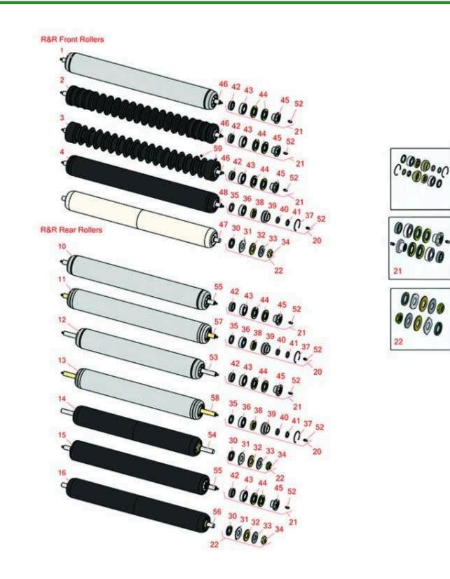
Replaces Toro Reelmaster 5410-D Parts DPA Cutting Unit with 7" Reel - Models 03681, 03682, 03696 & 03697 Front Rollers
